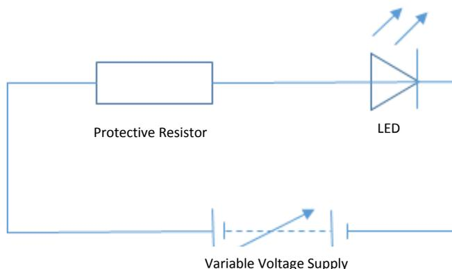
Notice that the LED will not light if the connections from the supply are reversed. Increasing the voltage (p.d.) across the LED results in increased brightness. The LED will light with only a small current.
